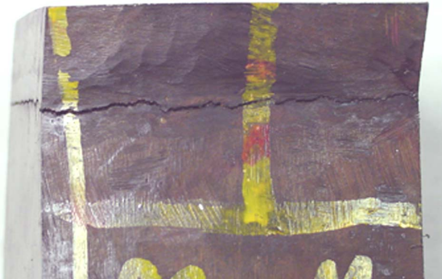
Figure 4-61 – Crack at weld from SS321 elbow shown in the Figure 4-60.
