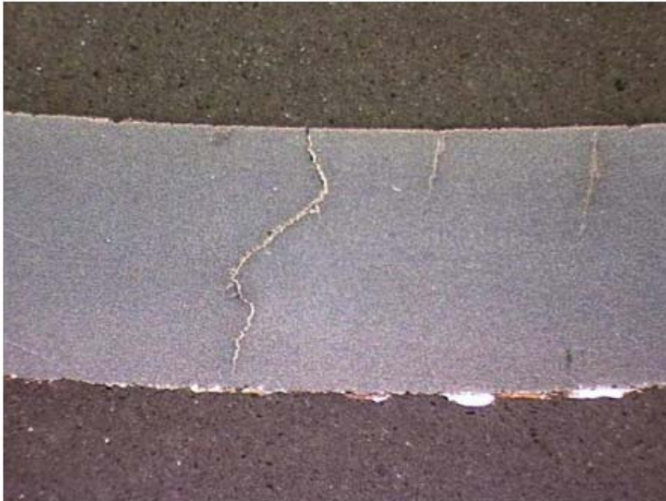
Figure 4-168 – Transverse cross-section of a piping section exposed to fuel ethanol showing multiple crack initiation sites characteristics of SCC.
