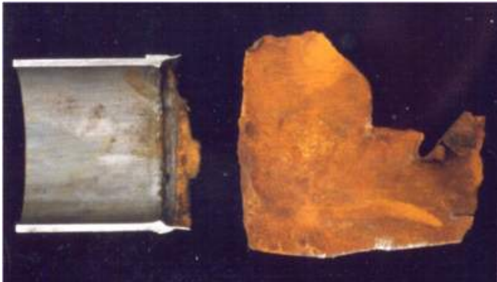
Figure 5-13 – Ruptured NPS 3 Sch. 80 0.216 in (5.49 mm) Depropanizer Feed Line operating <120°F Residual element content is as follows: Both Base metals: %C > 0.18 & %Cu + %Ni < 0.15 Weld Metal: %Cu + %Ni + %Cr < 0.15
