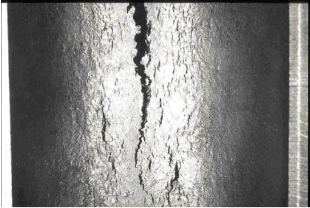
Figure 4-18 – Creep rupture of an HK40 heater tube.
