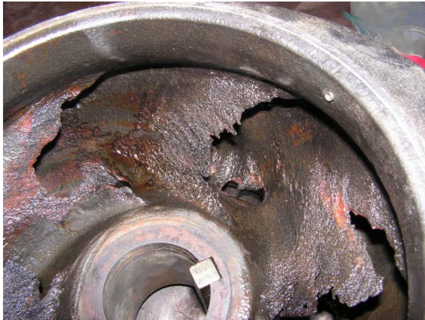
Figure 4-45 – Erosion-Corrosion of is ASTM A48 Class 30 Cast Iron Impeller in recycle water pump.
