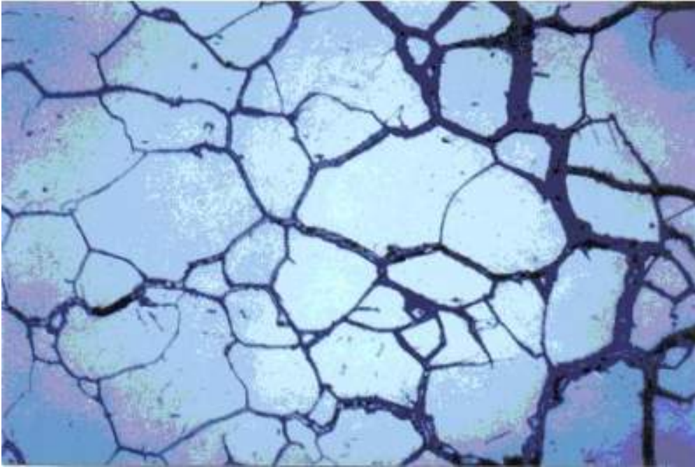
Figure 5-28 – Higher magnification view showing intergranular cracking. Mag. 200X.
