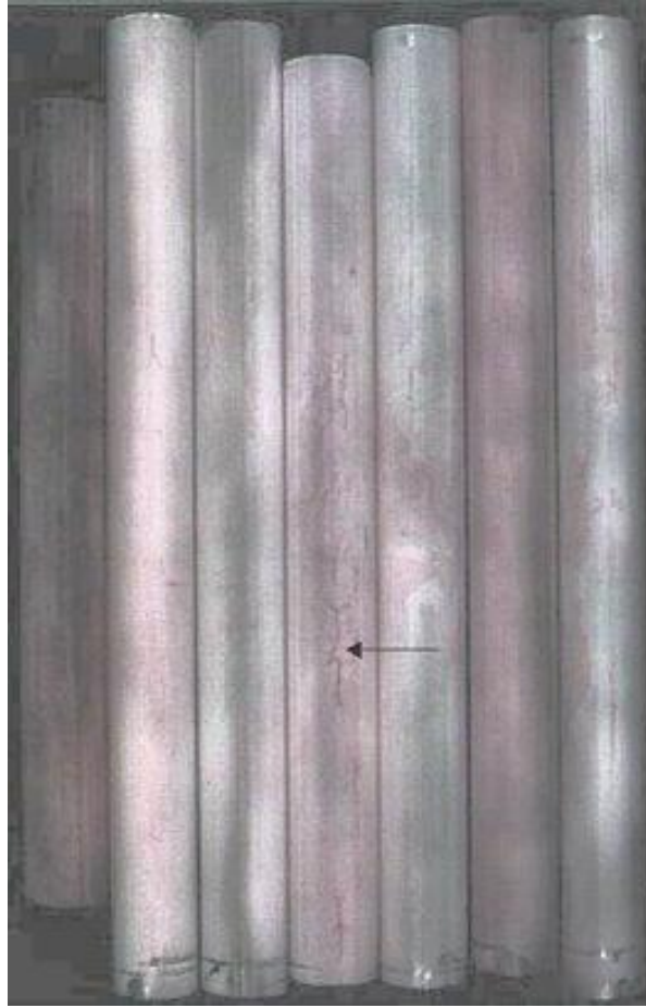
Figure 4-135 – Cracking on the shell side of Type 316L SS tubes in steam service at 450°F (232°C), showing tubes after PT inspection. The cracks can be seen in the center tube (arrow).
