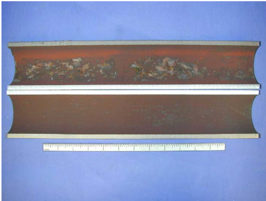
Figure 4-99 – I.D. deposits on CS boiler tube with damage due to caustic corrosion.
