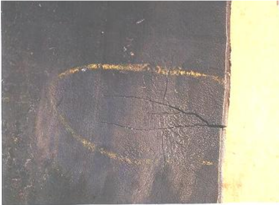
Figure 4-159 – Liquid metal embrittlement of Monel caused by mercury in an FCC gas plant overhead drum.
