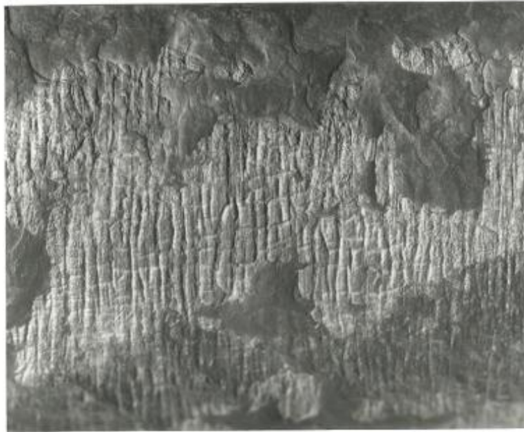
Figure 4-127 – The “alligator hide” morphology of liquid coal-ash corrosion is evident when the dense, glassy deposit is removed. Mag. 2.4X
