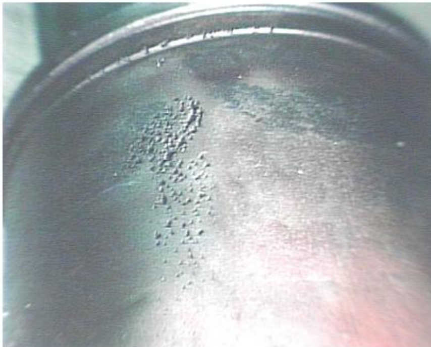
Figure 4-49 – Cavitation pitting on the water side of a cast iron cylinder liner in a large engine.
