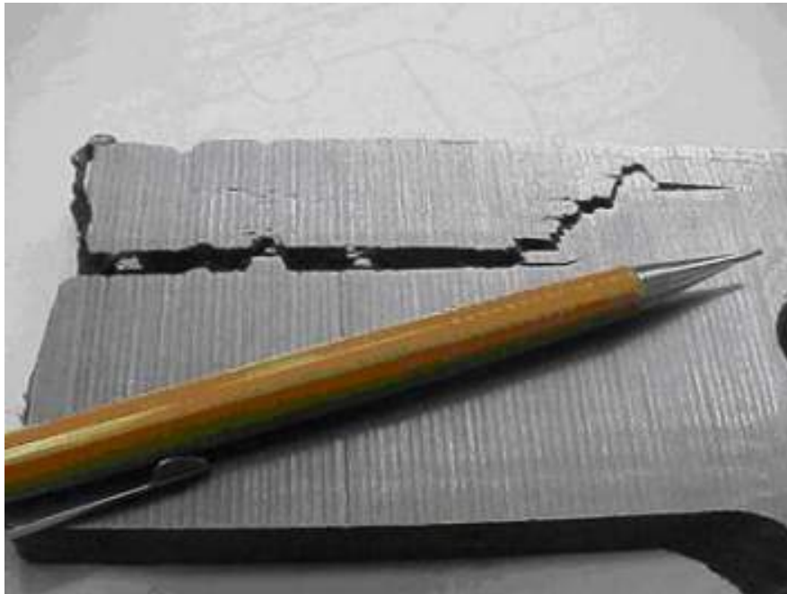
Figure 5-36 – Cross-section of plate showing HIC damage in the shell of a trim cooler which had been cooling vapors off a HHPs vessel in a hydroprocessing unit.
