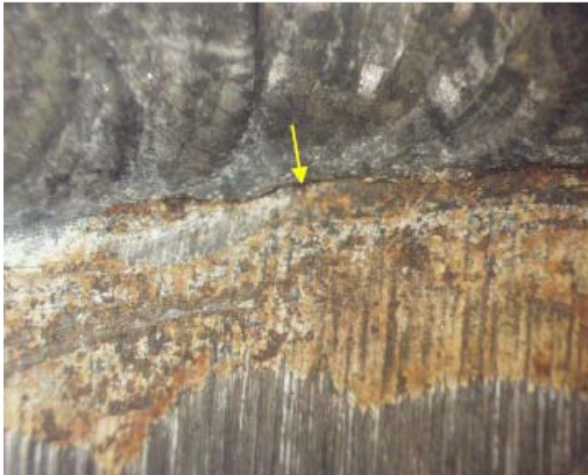
Figure 4-36 – Weld detail used to join a carbon steel elbow (bottom) to a weld overlaid pipe section (top) in high pressure wet H 2 S service. Sulfide stress cracking (SSC) occurred along the toe of the weld (arrow), in a narrow zone of high hardness.
