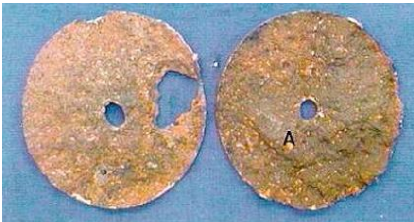
Figure 4-97 – Coupons removed from the bottom of an unprotected steel condensate storage tank after 3 years of service. The external surface is shown.
