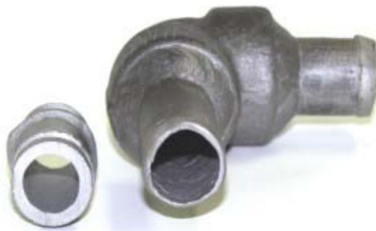
Figure 4-119 – Sulfidation failure of carbon steel sight glass nipple on the right after 2 years in crude unit. Original thickness is shown on left for comparison. Material was supposed to be 9Cr-1Mo.
