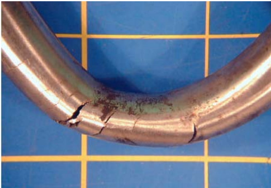
Figure 4-133 – External cracking of Type 304SS instrument tubing under insulation.
