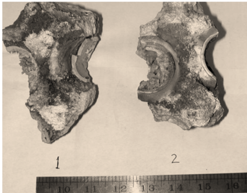
Figure 4-59 – Damaged refractory and ferrules.
