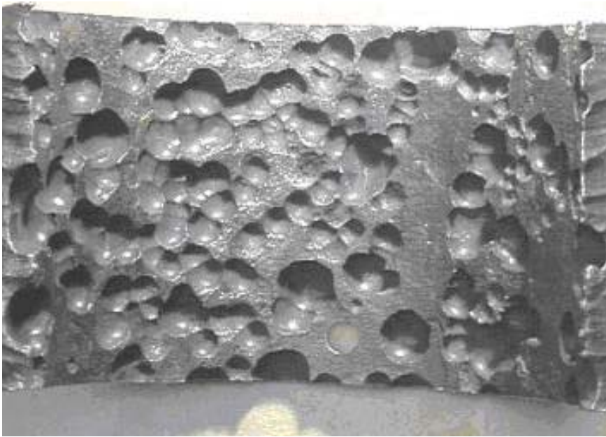
Figure 4-125 – Metal dusting of a 304H stainless steel pipe.
