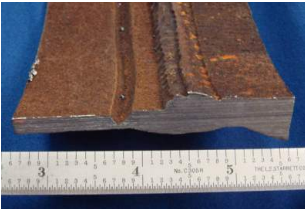
Figure 5-2 – Hot Lean Amine Corrosion of Carbon Steel:
