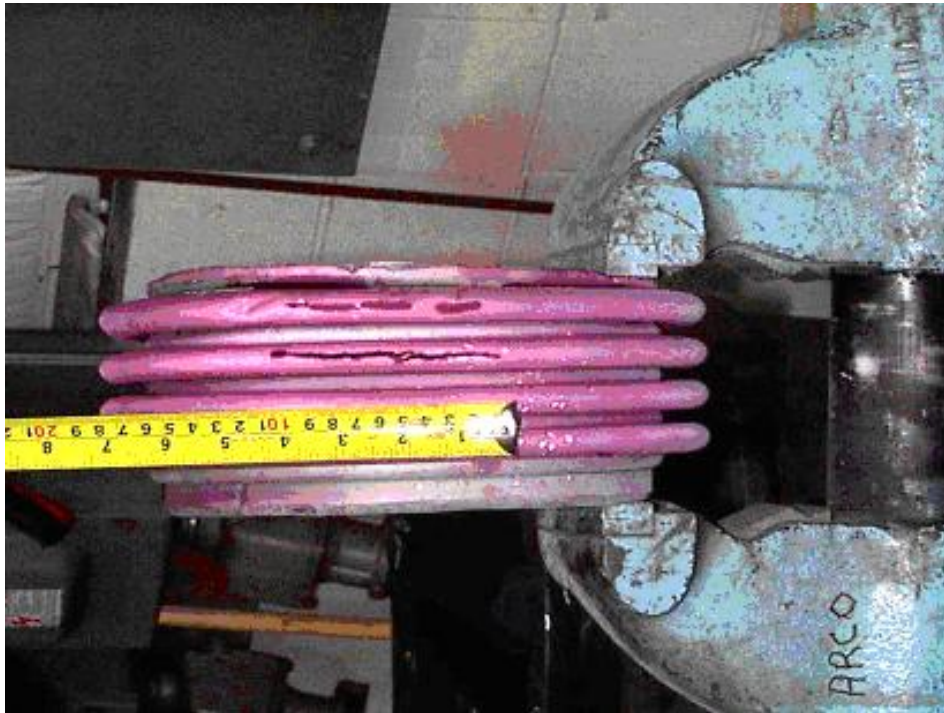
Figure 4-153 – Stainless steel expansion bellows from a steam-driven turbine previously subjected to a caustic carryover upset condition.
