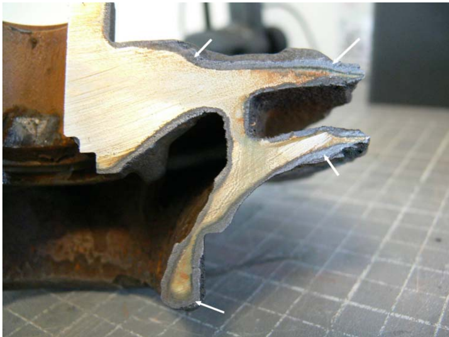
Figure 4-104 – Cut away of cast iron impeller shown above. The dark phase around the outside perimeter (at arrows) is graphite which surround the unaffected metal in the middle.
