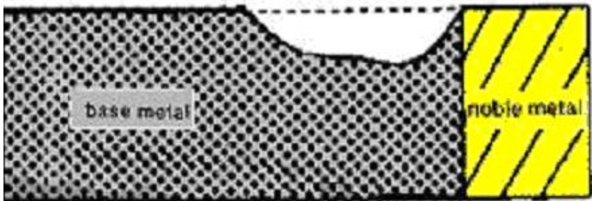
Figure 4-70 – Preferential galvanic corrosion of the more active component of the two materials.
