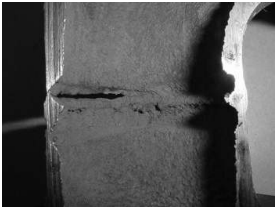
Figure 5-15 – Accelerated corrosion in the heat affected zone of a carbon steel weldment. Residual element content is as follows (Reference 8): Both Base metals: %C > 0.18 wt. & %Cu + %Ni < 0.15 Weld Metal: %Cu + %Ni + %Cr < 0.15
