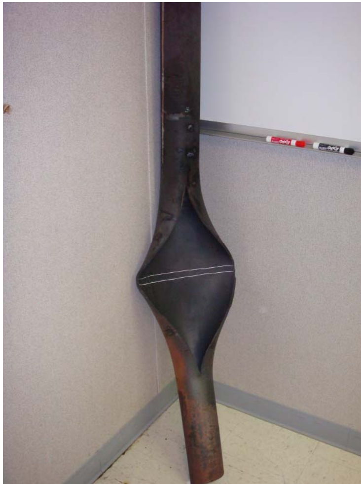
Figure 4-28 – Short term overheating failure of a vertical 4.5-in. OD, Schedule 160 2.25Cr-1Mo (SA335-P2) hydrocracker radiant that was 21 years old. Failure occurred due process side starvation with burners running.
