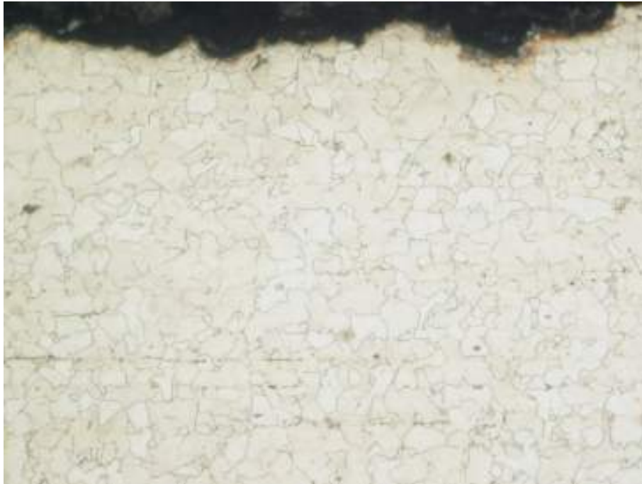
Figure 5-59 – A photomicrograph at the pipe ID surface exhibiting of the pipe shown in the previous pictures, exhibiting complete decarburization of the original structure. Mag. 200X
