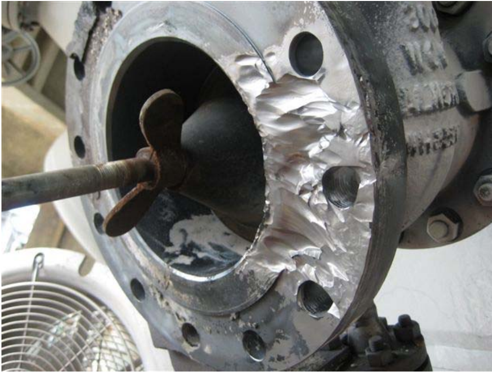
Figure 4-43 – Erosion Corrosion of a 1.25Cr 300 # valve flange on an FCC Catalyst withdrawal line.
