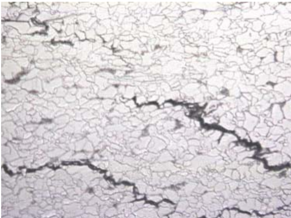
Figure 4-167 – The top picture shows cracking initiating in the base metal on the ID of a section of piping adjacent to the weld. The bottom picture is a high magnification photomicrograph of the crack above illustrating the predominately intergranular nature of the cracking. (380X – Nital etch)
